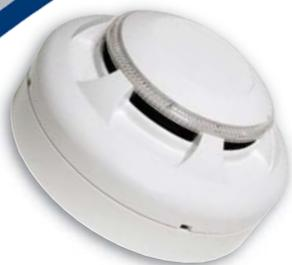
ii) Introduce a discrete amount of smoke into the detector head, e.g. using a 'No Climb -Solo' smoke test head. Check that the detector gives an alarm condition within 15 seconds. Check the LED indicator on the EVC-P detector illuminates and any remote indicator LED fitted also illuminates.
