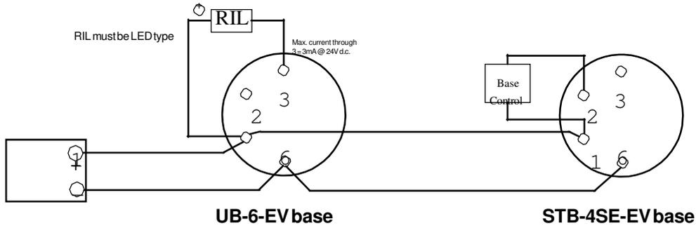
Auxiliary terminal RIL current limited to 3mA. Base control is not current limited as the auxiliary equipment provides the limiting. If the +ve supply for the auxiliary equipment is taken from the EV loop, care must be taken to not cause corruption of the EV protocol by excessive current draw.
