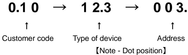
The 7 segment LED distinguishes the Customer Code, Type and Address by the dot position in the LED.
