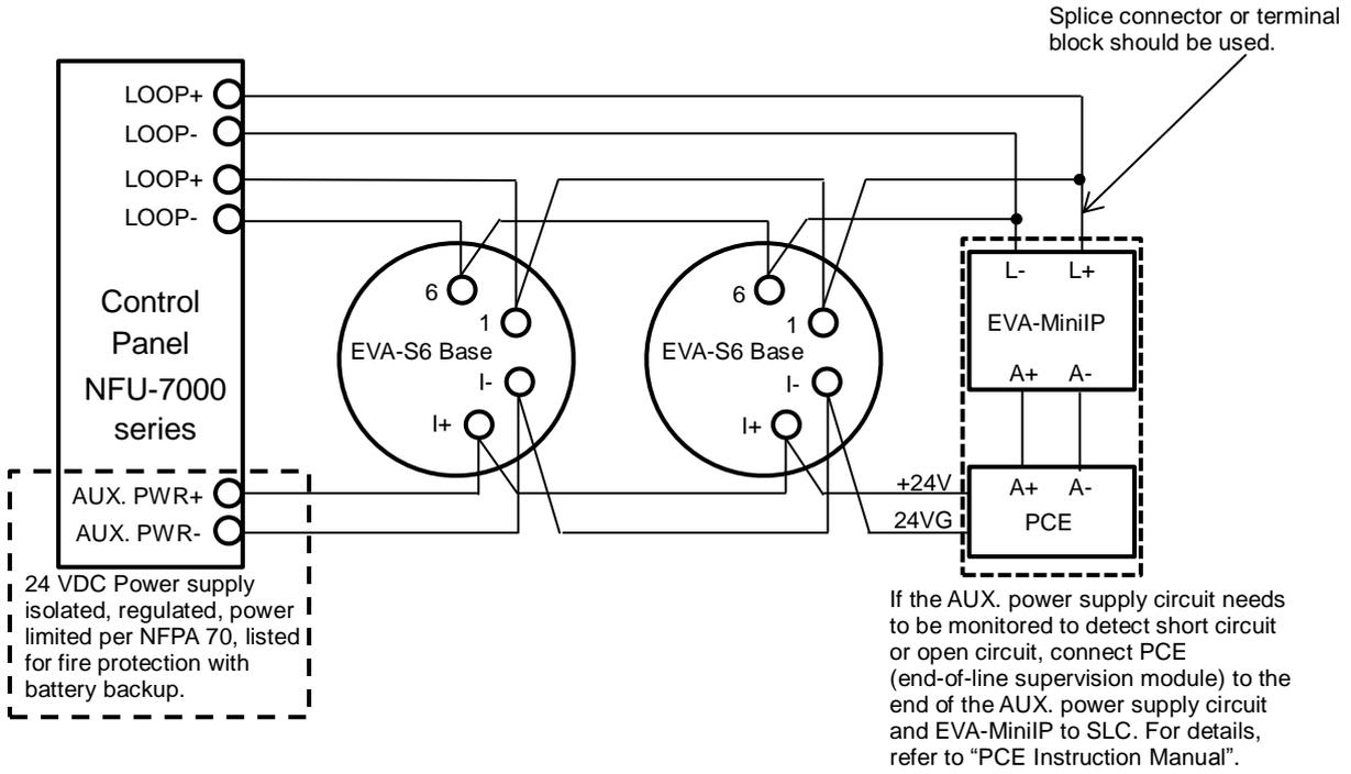
**Figure 5: Connection to control panel NFU-7000 series**
