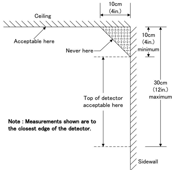
**Figure 5: Detector placement near ceiling or wall joints**
