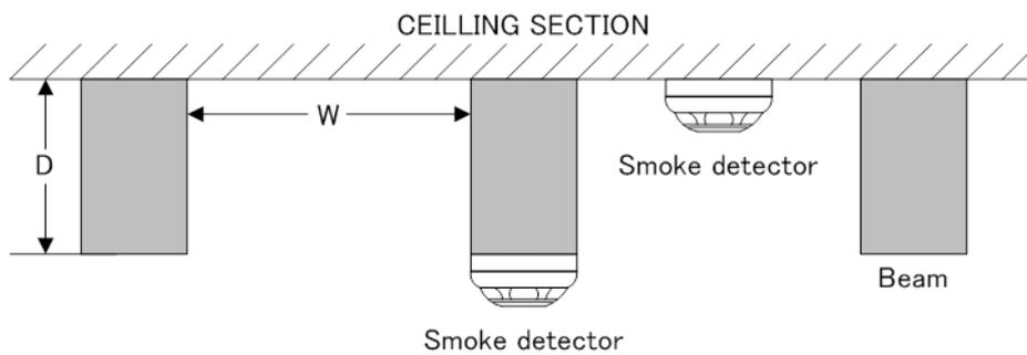
Figure 16: Smoke detector spacing — beam construction (side view)
