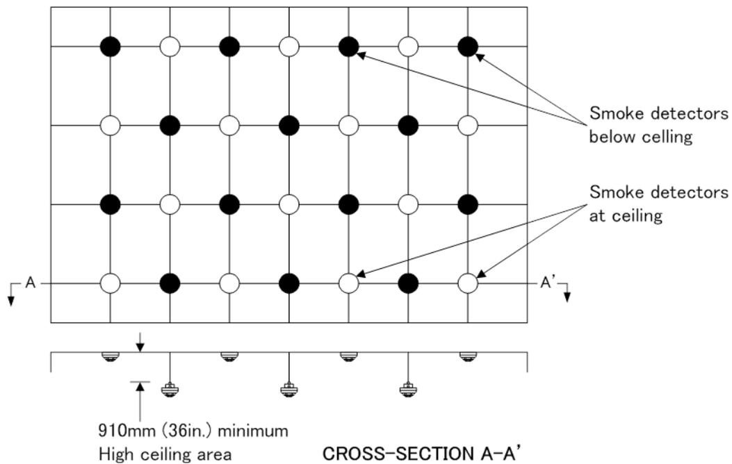
**Figure 13: Smoke detector layout accounting for stratification**
