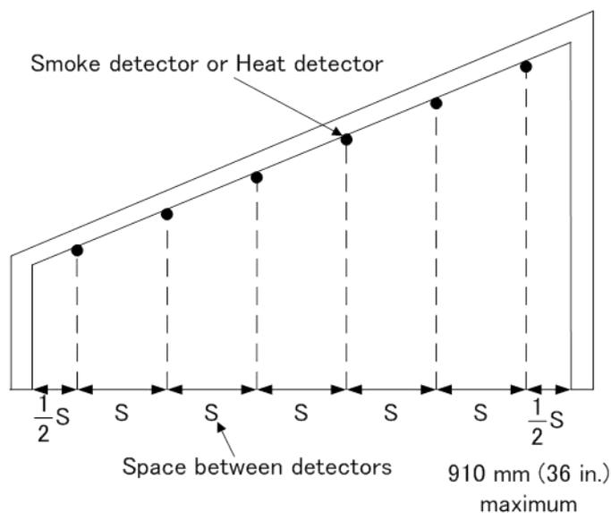
**Figure 12: Heat detector spacing — Sloped ceiling (shed type)**
