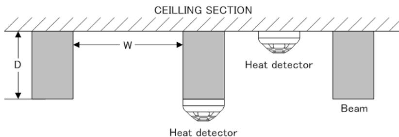
**Figure 9: Heat detector spacing — beam construction (side view)**
