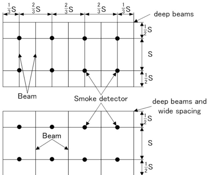
Figure 17: Smoke detector spacing — beam construction (plan view)
