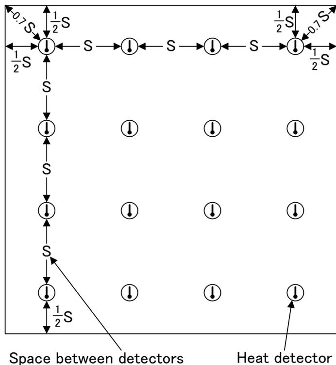
(1) Heat detector; S = Listed spacing between detectors
